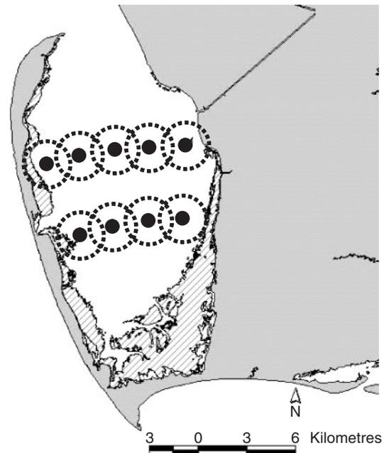
**Fig. 5.** Example of a study site with an acoustic array deployed in parallel curtain format where individual points indicate acoustic receiver placement. This configuration helps define whether fish have passed through one receiver line and provides information on directionality of movement. Dashed circles represent the detection range of each receiver.
