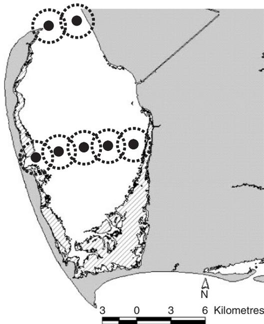
**Fig. 3.** Example of a study site with an acoustic array deployed in gate (upper) and curtain (lower) formats where individual points indicate acoustic receiver placement. Dashed circles represent the detection range of each receiver.
