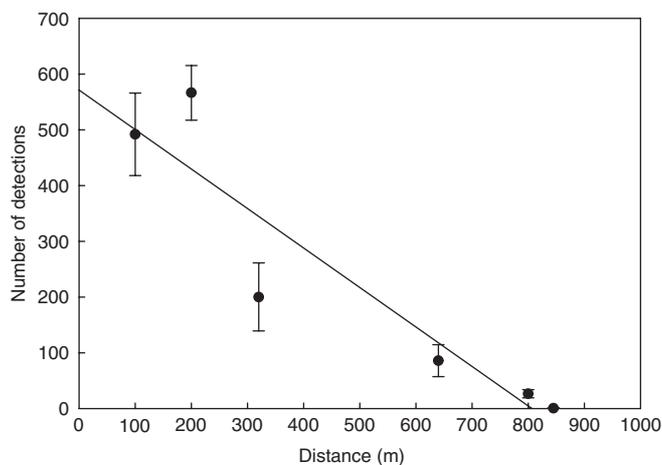
**Fig. 7.** Detection data from deployment of six acoustic transmitters for range testing in a Florida estuary. Transmitters were moored variable distances from each target receiver and the mean number of detections over one week for each transmitter is shown here. Bars indicate standard error and the line represents a linear regression ( $r^2 = 0.8589$ ) (M. R. Heupel, unpublished data from Charlotte Harbor, Florida).
