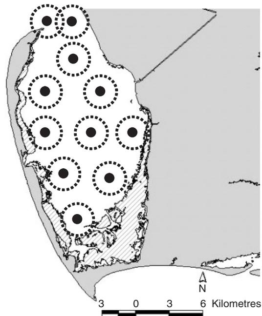
**Fig. 2.** Example of a study site with an acoustic array deployed in a 'fisheries' format. This system uses a grid layout, but does not require detection range overlap and allows receivers to be widely spaced. Individual points indicate acoustic receiver placement with dashed circles representing the detection range of each receiver.
