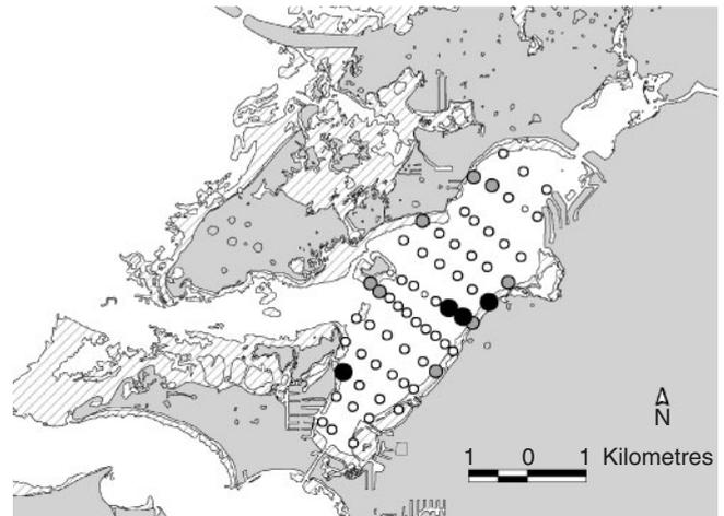
**Fig. 6.** Map of the Terra Ceia Bay (Florida, USA) study site showing the results of noise surveys at 69 kHz. Noise level was rated from 1 to 4 based on signal strength of background noise heard on the receiver where 1 = small open circle, 2 = larger open circle, 3 = small grey filled circle and 4 = large solid black circle. The two noisiest regions were due to an oyster reef and jetty pilings covered with barnacles and oysters (M. R. Heupel, unpublished data).
